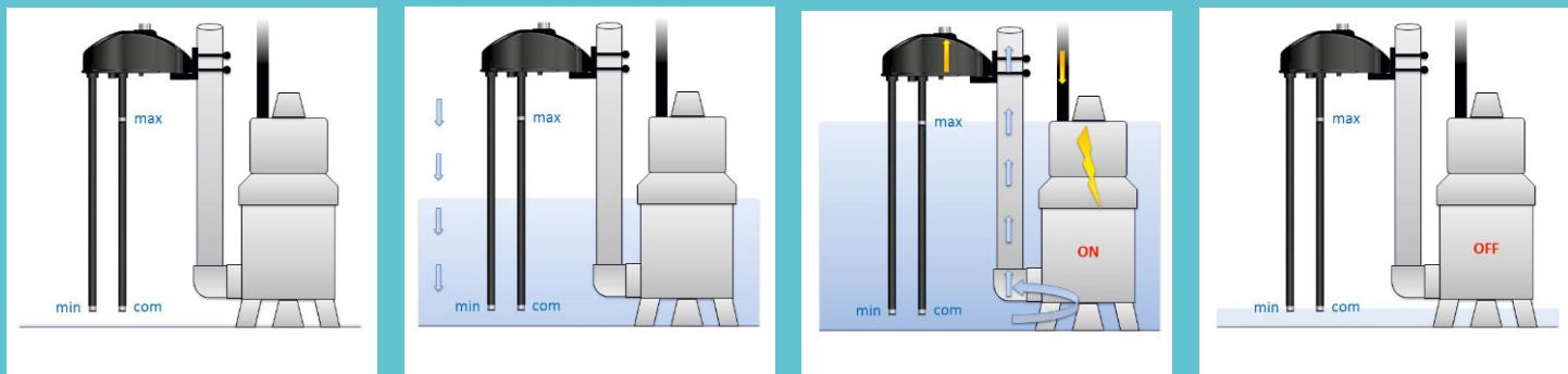
Spider is connected to 3 batons: Common as ground - Min as minimum level - Max as maximum level
