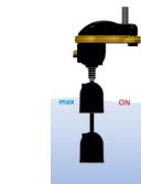
High level starts the pump and the tank drains
